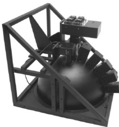
Figure 13: The Imaging Sphere IS-SA with Prototype Fixed Illumination Positions
