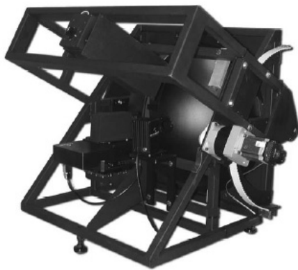
Figure 12: The Imaging Sphere IS-SA for Surface Scatter Testing with Adjustable Illumination Direction
