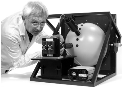
Figure 5: The Original Philips Parousiameter with its Inventor, Sipke Wadman
