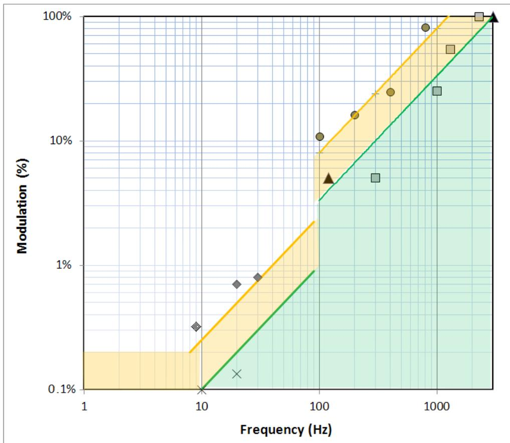
Figure 3 - Graph showing low risk (yellow) and NOEL (green) modulation percentage against frequency [3]. The data points on this graph relate to data from research into visible flicker (diamonds [8, 9]), stroboscopic effects (squares [10] and circles [11]) and phantom arrays (triangles [12])
