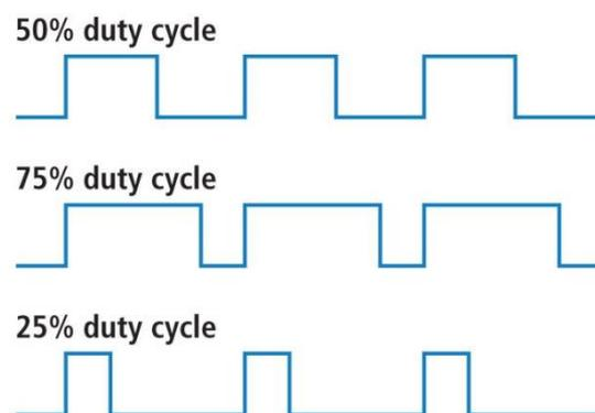
Figure 2 - Pulse width modulation (PWM) waveform [13]
