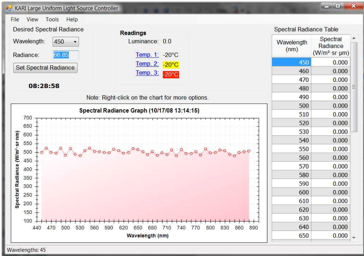
Figure 4. Automatic mode display window for the system control software
